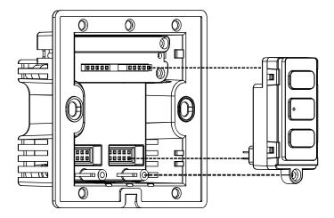
During installation of the modules, care should be taken to ensure that the connecting pins are lined up and straight before fully inserting. Please DO NOT continually remove and install the modules.
