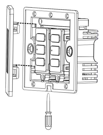
Removing the faceplate can be done using a small 4-6mm flat blade screwdriver.
