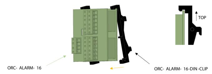
2. Connect the DIN bracket at the top of the Din Rail, then push back the DIN bracket at the bottom "Click"
