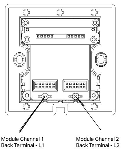
Maximun load: Switch Module = 150W / Dimmer Module = 150W
