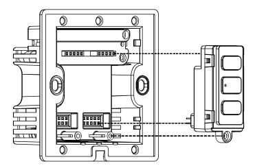
During installation of the modules, care should be taken to ensure that the connecting pins are lined up and straight before fully inserting. Please DO NOT continually remove and install the modules.
