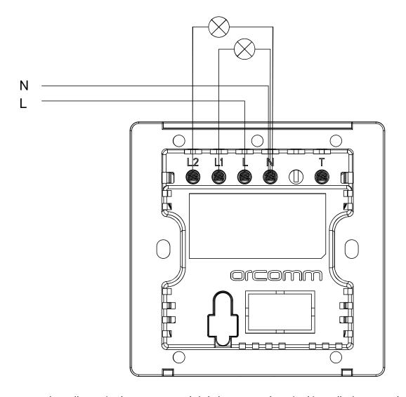
Please ensure that all terminals are secured tightly as per electrical installation standards.
