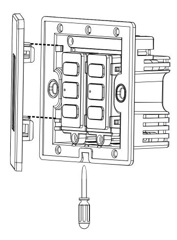
Removing the faceplate can be done using a small 4-6mm flat blade screw driver.
