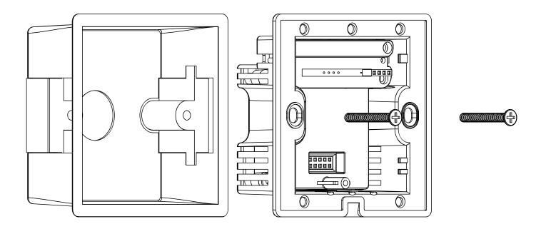
Once connections and terminations are complete, secure with the provided M3.5mm PH2 drive screws.
