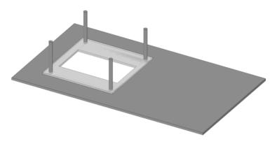
Pass cable through hole and mount bracket on rear of reader
