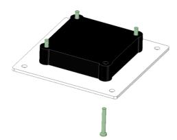
Line the reader holder up with the outer Studs and secure with washers and nuts.
