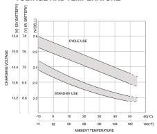
Fast constant current bulk charge 3 stage charging CI-CV-float Constant voltage float/standby Proportional timing Flexibility, to match battery specification.
