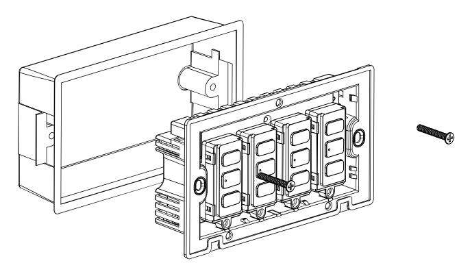
Once connections and terminations are complete, secure with the provided M3.5mm PH2 drive screws.
