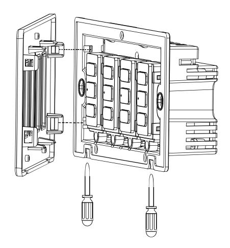
Removing the faceplate can be done using a small 4-6mm flat blade screw driver.
